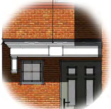
Flat portico with wood grain and rolled lead effect top. Individual formal 6 panel styled front door with ironmongery letterbox.
