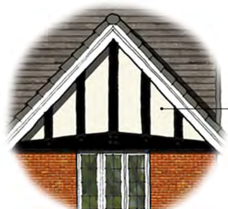
Black tudor board with fixing pegs on chalk render
