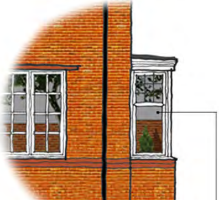
Square bay with lead rolled top roof
