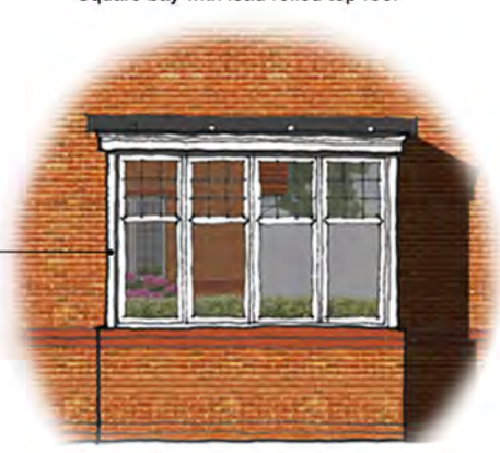
Square bay with lead rolled top roof
